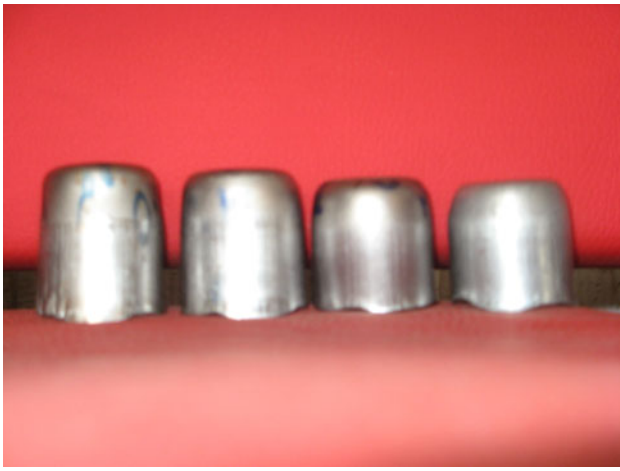
Fig. 5 Successfully deep drawn cups from 1.2 mm thick sheet with different draw ratios using hydromechanical deep drawing
