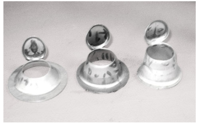
Fig. 7 Typical failures observed in hydromechanical deep drawing
