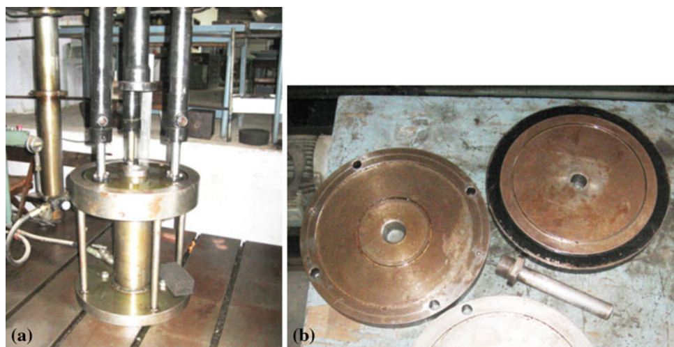
Fig. 2 Experimental setup used for hydromechanical deep drawing experiments. (a) Pressure chamber and the blank holding system and (b) tools (Dies and Punch)
